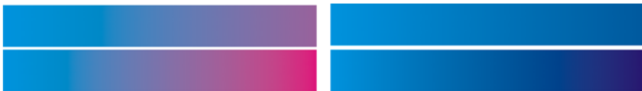
Figure 13: CMYK Magenta is added (left). Blue (C100, M100, Y0, K0) is added (right).
